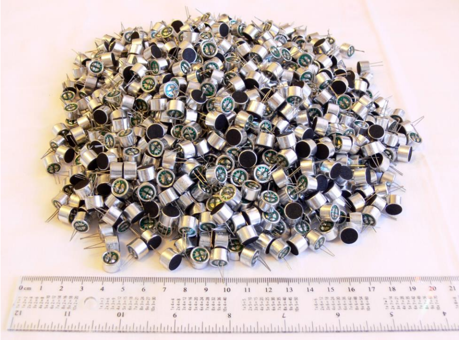
Fig. 1. BAT Vision uses microphones for its two-level hierarchical acoustic array
